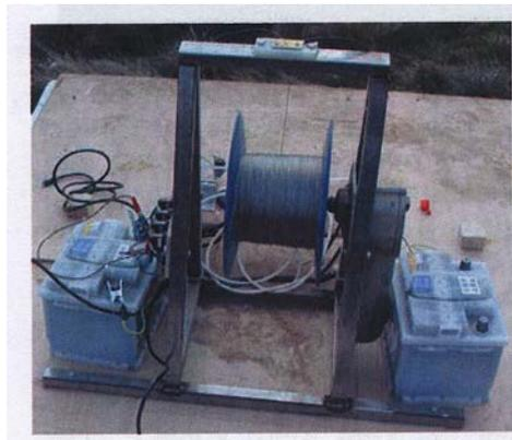
After that it really got interesting. The kite continued to fly well at about 130m. The line (wire) came from a powered drum fixed on a thick polystyrene base (see Photo) with a beautifully built Perspex cover
